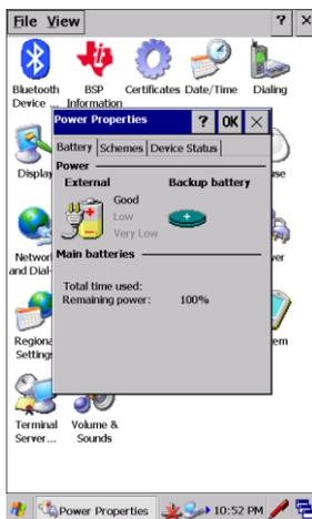
In the schemes user can change adjust the time to switch state to User Idle, System Idle, or Switch to suspend. The other Device Status tab shows the power level for each device such as COM, OTG and so on
