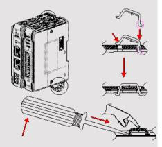
Rail mounting: DIN rail 35mm.
