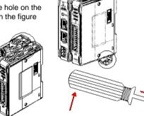
Rail mounting: DIN rail 35mm.
