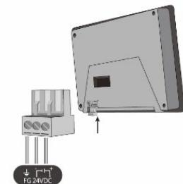
**NOTE: Connect positive DC line to the '+' terminal and the DC ground to the '-' terminal.**
