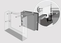
Plan for adequate space around the unit and inside the enclosure, for ventilation and cables. Consider the heat from other devices inside the enclosure. The ambient temperature around the unit must be  $0 \sim 50^{\circ}$ C
