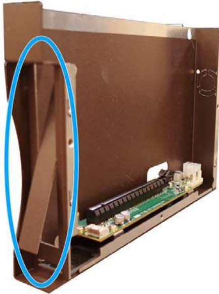
Remove bezel cover and insert the card
