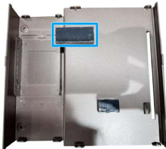
Nuvo-11000E series bottom panel's thermal pad
