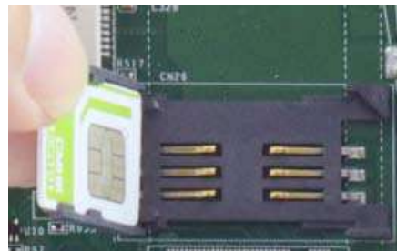
Insert Mini-SIM card with pins facing up
