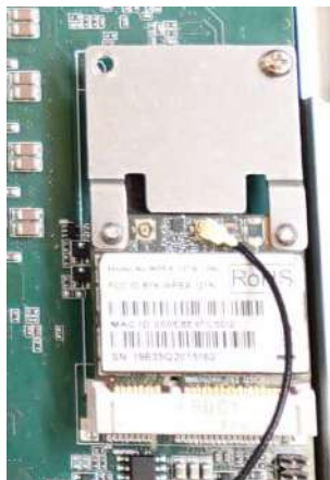
Clip on IPEX-to-SMA cable Secure antenna to rear panel
