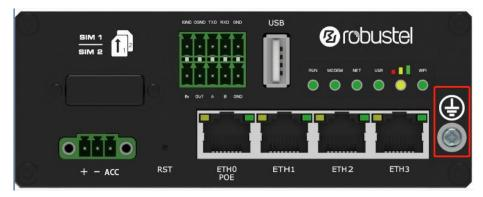
Router grounding helps prevent the noise effect due to electromagnetic interference (EMI). Connect the router to the site ground wire by the ground screw before powering on.
