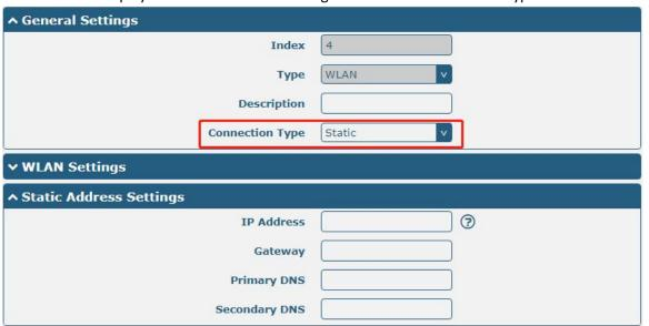
R2110 does not support the **PPPoE** WLAN Connection Type.
