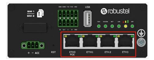
There are four Ethernet ports on R2110-4L, including ETH0 (POE), ETH1, ETH2, ETH3. Each has two LED indicators. The yellow one is a link indicator but the green one doesn't mean anything. For details about status, see the table below.
