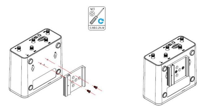
Use 3 pcs of M3\*8 Black cross recessed countersunk head tapping screws to mount the router on the DIN rail, and then hang the DIN rail on the holder. You need to choose a standard holder.
