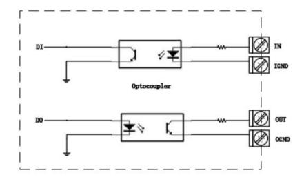
R1520 supports 1 channel DI and 1 channel DO, the internal schematic diagram is as shown above;
