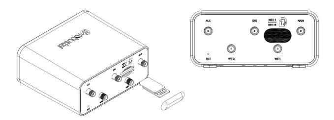
Insert or remove the SIM card as shown in the following steps.
