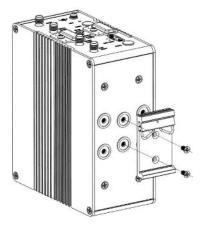
**6. Wall Mounting.** Use 4 M3 screws to fix the DIN rail to the device, then hang the DIN rail on the mounting bracket.
