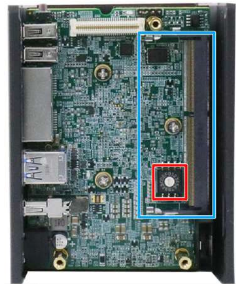
DRAM slot and ignition switch
