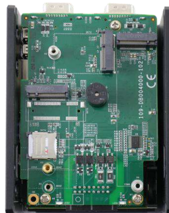
Secure micro SIM with cover
