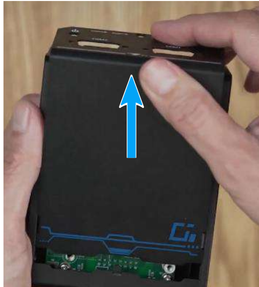
Slide open the L-shape panel
