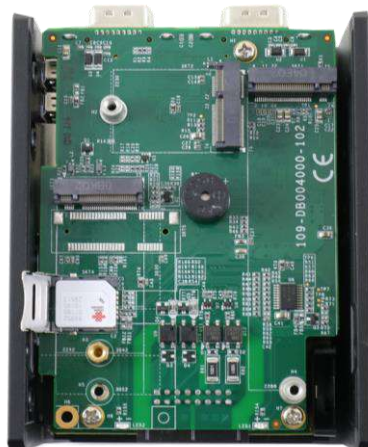
Place micro SIM in slot
