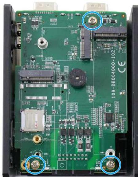
Remove the screws
