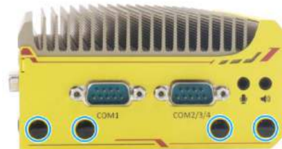
COM port panel antenna openings
