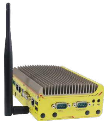
Attach external antenna
