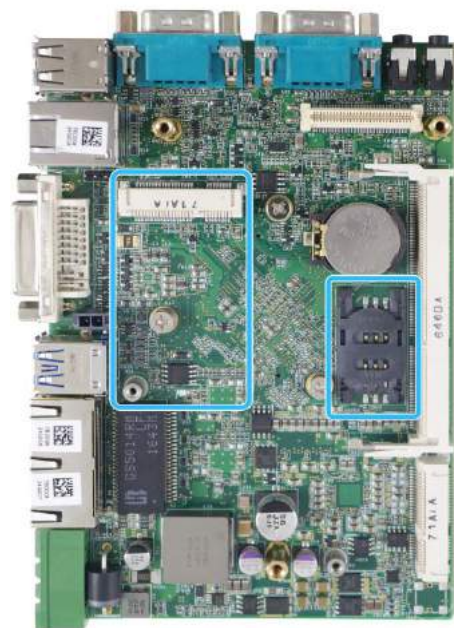
mini-PCIe/ SIM slot on the mainboard
