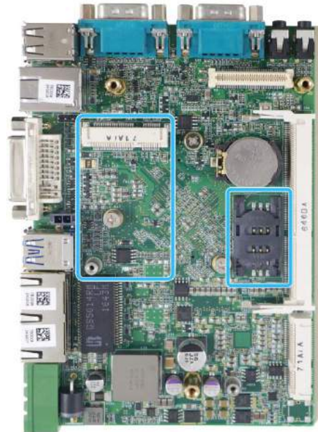
mini-PCIe/ SIM slot on the mainboard
