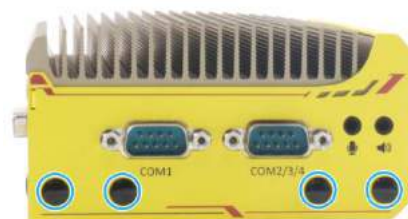
COM port panel antenna openings
