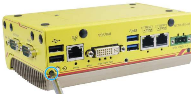
Screw next to the power button on the front panel
