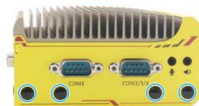
COM port panel antenna openings
