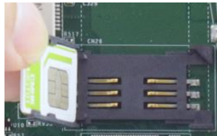
Insert Mini-SIM card with pins facing up
