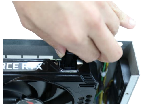
Unplug the 8-pin power cable
