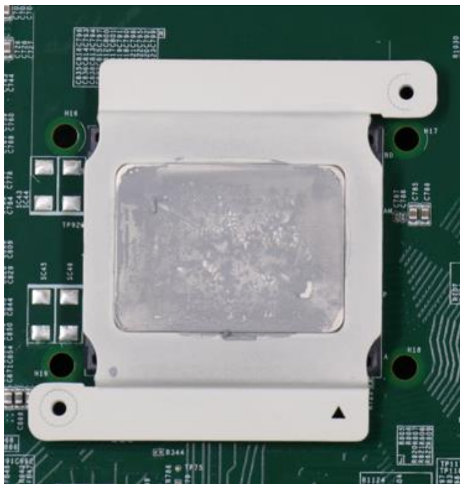
CPU retention bracket (holder)
