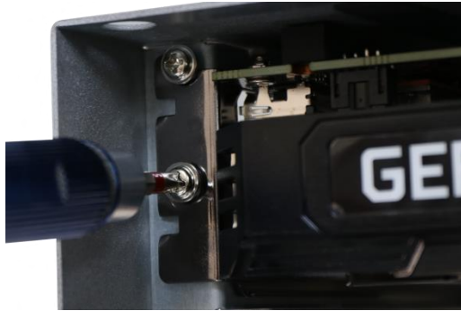
Remove the screws securing the graphics card
