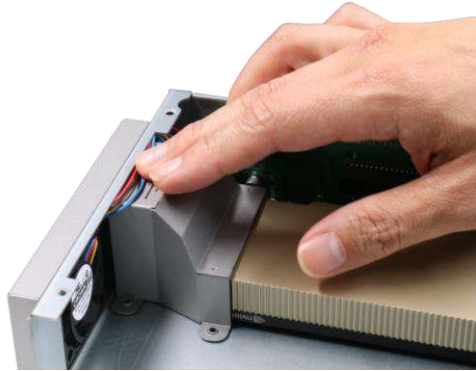
Reinstall the duct
