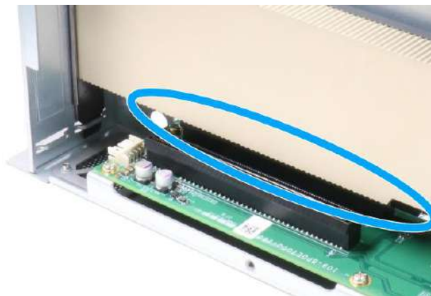
Properly inserted into the PCIe slot
