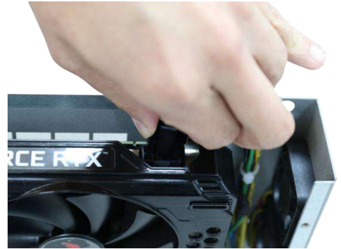
Unplug the 8-pin power cable
