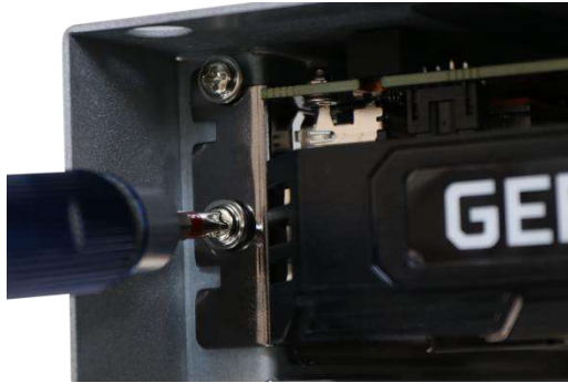
Remove the screws securing the graphics card
