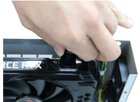
Connect the 8-pin power cable
