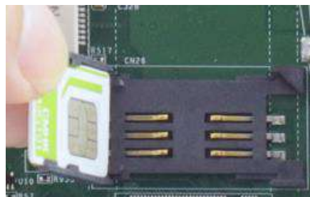
Insert Mini-SIM card with pins facing up
