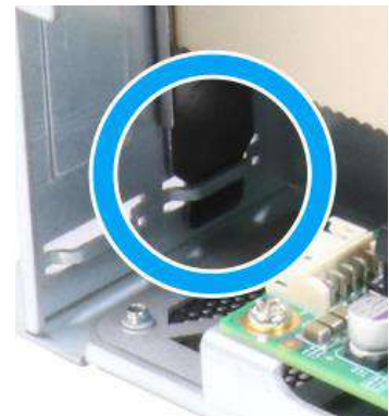
Bezel inserted into the notch
