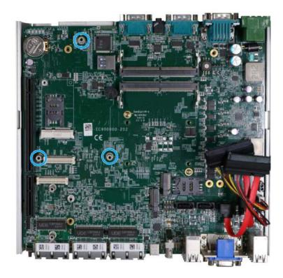
3. Gently lower the MezlO<sup>TM</sup> module onto the three stand-mounts while matching the MezlO<sup>TM</sup> interface. Secure the module using three screws supplied.
