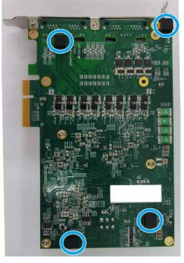
Rubber stands, remove each protective film (indicated in **red**) before attaching to the card
