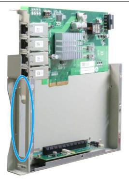
Remove bezel cover and insert the card
