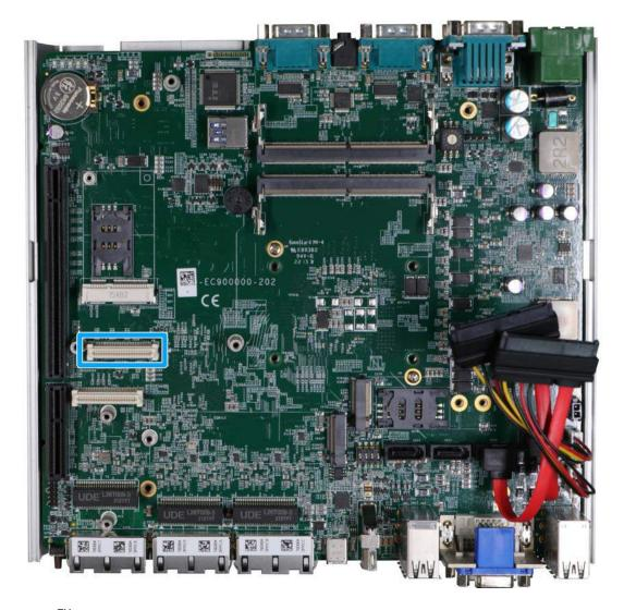
MezIO<sup>TM</sup> is an innovative interface designed for integrating application-oriented I/O functions into an embedded system. It offers computer signals, power rails and control signals via a high-speed connector. MezIO<sup>TM</sup> is also mechanically reliable benefited from its 3-point mounted mezzanine structure. A MezIO<sup>TM</sup> module can leverage these signals to implement comprehensive I/O functions.
