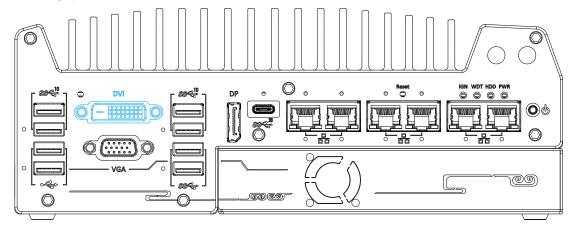
DVI-D transmits graphics data in digital format and therefore can deliver better image quality at high resolution. The DVI connector on the front panel can either output DVI signals or other digital signals (via an adapter/ cable) depending on the display device connected. It supports resolutions up to 1920x1200@60Hz.
