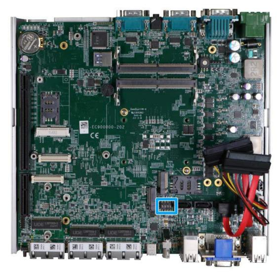
The DIP switch (indicated in **blue**) should be already configured out of the factory. Users need only set the 4th DIP switch to ON for BIOS update and switch it back to the OFF position when BIOS upgrade has completed. The table below shows the system default DIP switch settings for reference purposes.
