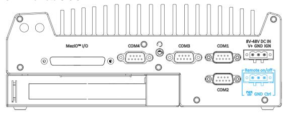
The "Remote On/ Off" 3-pin connection allows for the connection of an external non-latched switch to turn on/ off the system. It is useful when the system is placed in a cabinet or a not easily accessed location. You may connect an external status LED (20mA) indicator by connecting to PWR LED and GND.
