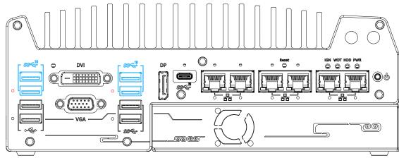
The system's USB 3.2 Gen2x1 ports (10Gbps) are implemented via native xHCI (eXtensible Host Controller Interface) controller and are backward compatible with USB3.2 Gen.1 USB 2.0, USB 1.1 and USB 1.0 devices. UFEI USB is also supported so you can use USB keyboard/mouse in UEFI shell environment. Indicated in **red** are screw-lock holes for the corresponding USB port.
