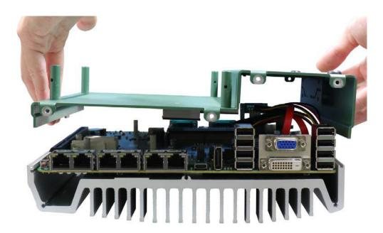
8. Once the bottom panel has been removed, you should have access to the system's internal I/O interfaces.
