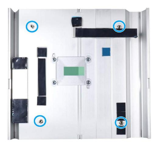
11. Once the motherboard has been installed, you're ready to secure the four screws that help the heatsink apply pressure to the CPU/ chipset die. You'll want to apply even pressure to the corners by gradually tightening each screw. Please refer to the recommended order when tightening the screws.
