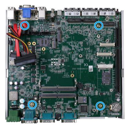
Secure motherboard with four screws
