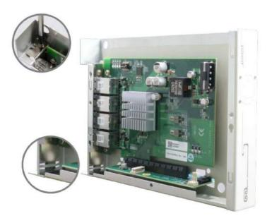
Make sure the card is inserted into the notch and secured with a screw
