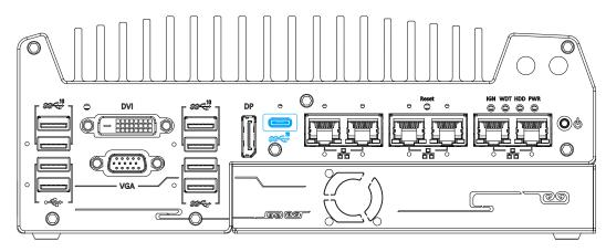
The system's USB 3.2 Gen2x2 type-C port offers up to 20Gbps of data transfer bandwidth, and is implemented via the native xHCI (eXtensible Host Controller Interface) controller. The port is backward compatible with USB3.2 Gen.1 USB 2.0, USB 1.1 and USB 1.0 devices via a USB hub (not included) to connect to external devices.
