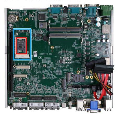
3. Before installing the mPCIe module, you need to insert the Mini-SIM card. Slide the SIM slot holder and lift the SIM card holder. Insert the Mini-SIM card (pins facing up), shut the SIM holder and slide it to lock the SIM card in-place.
