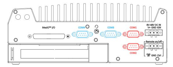
The system provides four COM ports for communicating with external devices. These COM ports are implemented using industrial-grade ITE8786 Super IO chip (-40 to 85°C) and provide up to 115200 bps baud rate.
