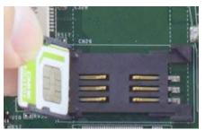
Insert Mini-SIM card with pins facing up
