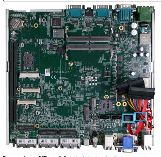
The system has two SATA ports (indicated in blue) and two four pin power connectors (indicated in red). The SATA and power cables should already be connected on the motherboard so users only need to install the HDD/ SSD. Please refer to the following instructions on how to install 2.5" SATA HDD/SSD.
