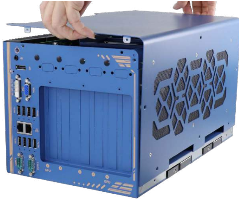
Place L-shape side panel onto the enclosure
