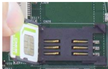
Insert Mini-SIM card with pins facing up
