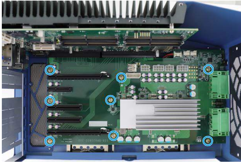
Remove screws securing the daughter-board
