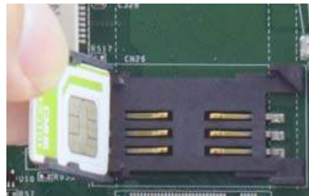
Insert Mini-SIM card with pins facing up
