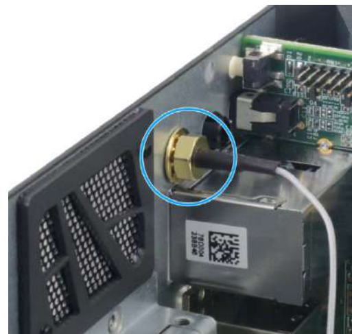
Secure antenna to rear panel
