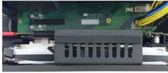
Graphics card stabilizing bracket
