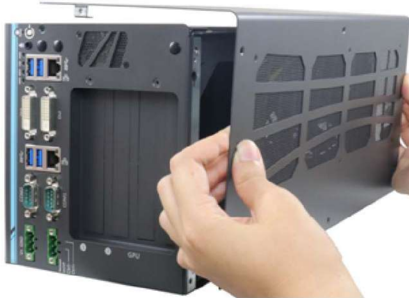
Place side panel onto enclosure
