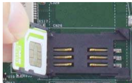
Insert SIM card with pins facing up
