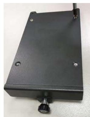
Secure the HDD
