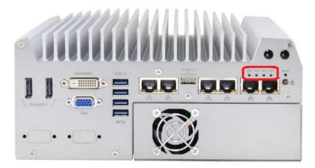
There are four LED indicators on the front panel: PWR, HDD, WDT, and IGN. The descriptions of these three LED are listed in the following table.
