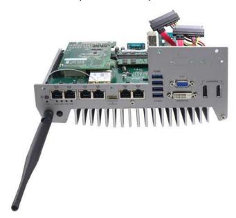
5. Recover the front panel, back panel and the bottom cover and attach a 3G antenna to the SMA connector. The mini-PCIe #2 socket shall be used in conjunction with the panel-accessible SIM socket on the back panel. Insert the SIM card upside down to the SIM socket to support 3G communication for your Nuvo-5095GC controller.
