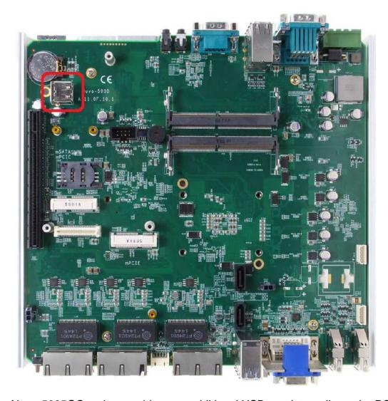
Nuvo-5095GC series provides one additional USB port internally on the PCBA. It supports standard USB 2.0 signals. You can utilize this USB port to connect a USB protection dongle inside the chassis of Nuvo-5095GC controller.
