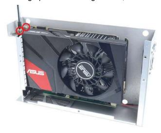
8. Recover the Cassette cover and fix it with three M3, flat-head screws. And put Expansion Cassette back to Nuvo-5095GC controller, and fix it using four M4 screws.
