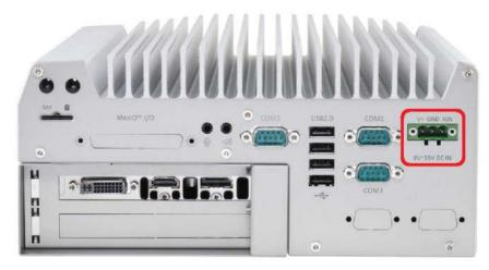
Nuvo-5095GC series allows a wide range of DC power input from 8 to 35V via a 3-pin pluggable terminal block, which is fit for field usage where DC power is usually provided. And the screw clamping connection of the terminal block gives a very reliable way of wiring DC power. For detail information of supplying DC power via pluggable terminal block, please refer to section 3.9.
