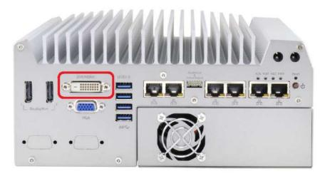
Nuvo-5095GC series has multiple display outputs on its front panel for connecting different displays according to your system configuration. DVI/HDMI transmits graphics data in digital format and therefore can deliver better image quality at high resolution. The DVI/HDMI connector on the front panel can either output DVI signals or HDMI signal depending on the display device connected. It supports up to 1920 x 1200 resolution. You can use a DVI to HDMI cable to connect a HDMI display device.
