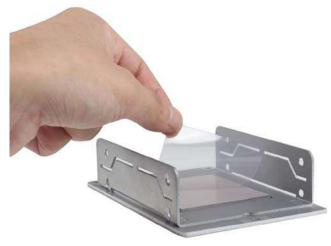
Place the HDD/SSD into the bracket and gently push it down to make it contact with the thermal pad. Use a Philips screwdriver to fix it with M3 flat-head screws from the accessory box. Please note that the HDD must be placed in the right direction as below.
