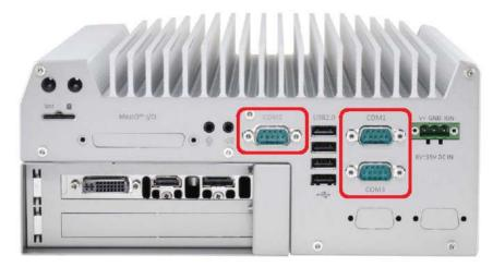
Nuvo-5095GC series provides three COM ports for communicating with external devices. COM1, COM2 and COM3 are located on the back panel via 9-pin D-Sub male connectors. They are implemented using industrial-grade ITE8786 Super IO chip (-40 to 85°C) and provide up to 115200 bps baud rate.
