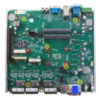
3. Gently lift the PCBA from the heat-sink. The CPU and CPU retaining bracket shall stay with the heat-sink.
