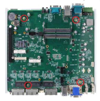
3. Place the PCBA on a flat surface. Remove the plastic protective cover from the LGA1151 socket.
