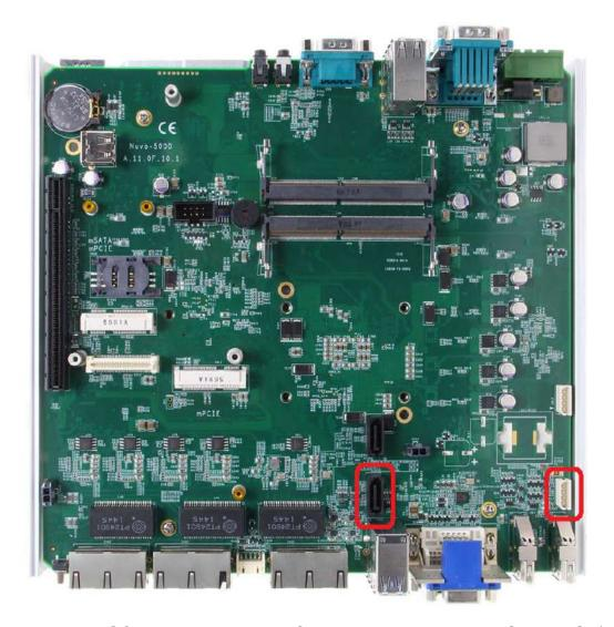
Nuvo-5095GC series provides two SATA ports which support Gen3, 6 Gb/s SATA signals. Each SATA port is composed of a 7-pin SATA connector and a 4-pin power connector. SATA port #2 is used in conjunction with the HDD bracket to accommodate the second 2.5" HDD/SSD. A dedicated cable is shipped with the system to provide standard 22-pin SATA connector. For information of installing a HDD/SSD to SATA port #2, please refer to section 3.4 for detail.
