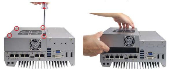
2. Open the cover of Cassette by loosening three M3 flat-head screws.
