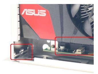
7. Fix the graphics card using two M3, PW-head screws.
