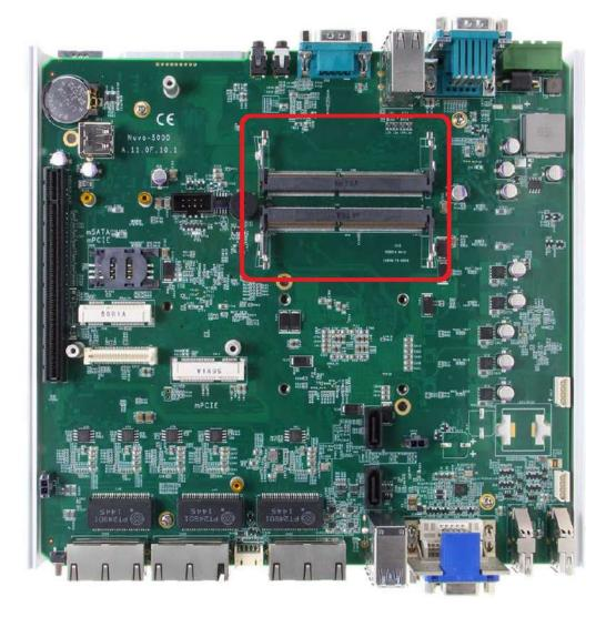
Nuvo-5095GC series provides two 260-pin, SODIMM sockets for installing DDR4 memory modules. It supports maximal 32GB capacity by installing two 16GB DDR4 2133 MHz SODIMM modules. For information of installing DDR4 memory modules, please refer to section 3.3 for details.
