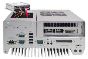
Place the HDD/bracket assembly back to the bottom cover. And fix it with three M3 5. flat-head screws.
