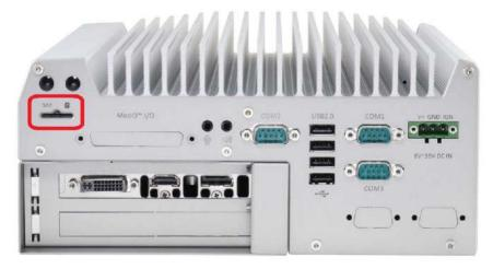
Nuvo-5095GC series provides a panel-accessible SIM socket is on the back panel. Combining with a 3G/4G module installed on internal mini-PCle port, you can have Internet access via telecom operator's network. The SIM socket is a push-push type. You can insert and push a SIM card to the end to install it, and push the installed SIM card again to eject it. Please note that SIM card must be inserted upside down. You can refer to section 3.5 for information of installing a 3G/4G module and SIM card.
