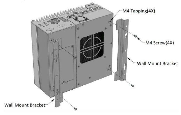
2. Place Nuvo-5095GC controller on a flat surface and fix it with screws. You can also take advantage of the keyhole-shaped holes of mounting brackets to suspend the Nuvo-5095GC controller on the Wall.
