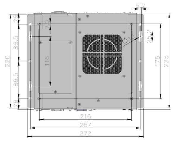
3. For the case of wall-mounting, please mount your Nuvo-5095GC controller in a right direction for better efficiency of heat dissipation.
