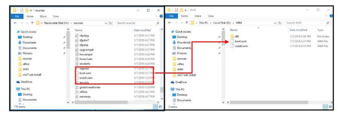
5. Copy the batch file (Win7\_USB3\_Patch\_x86.bat or Win7\_USB3\_Patch\_x64.bat) to D:\WIM. You can find the batch file in x:\Driver\_Pool\USB3\_10\_Series\Win7\_ALL.
