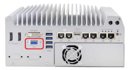
Nuvo-5095GC series has multiple display outputs on its front panel for connecting different displays according to your system configuration. VGA connector is the most popular way for connecting a display. The VGA output on Nuvo-5095GC series supports up to 1920 x 1200 resolution. By BIOS default and hardware implementation, the VGA output is always enabled even when VGA monitor is not connected.
