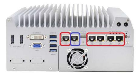
Nuvo-5095GC series offers 6 GbE ports on its front panel. The GbE port marked in blue is designed with Intel<sup>®</sup> I219-LM and ports marked in red are implemented with Intel<sup>®</sup> I210-IT Gigabit Ethernet controllers.
