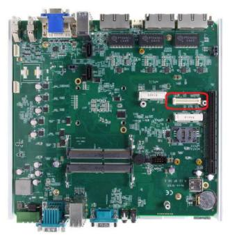
2. Align the board-to-board connector on the MezIO-C180 module to to connector on the PCBA. Gently push it down and make sure the connector is firmly contacted. Fix the MezIO<sup>TM</sup> module with three M3 P-head screws.
