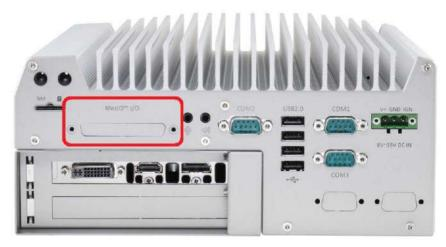
Nuvo-5095GC series incorporates Neousys' MezlO<sup>TM</sup> interface. You can install a MezlO<sup>TM</sup> module to expand application-oriented I/O function. To support MezlO<sup>TM</sup> I/O connectivity, Nuvo-5095GC series reserves the cutting hole for a SCSI-II 68-pin connector on its back panel. Please refer to section 2.5 for information of MezlO<sup>TM</sup> interface and section 3.6 for installing a MezlO<sup>TM</sup> module.
