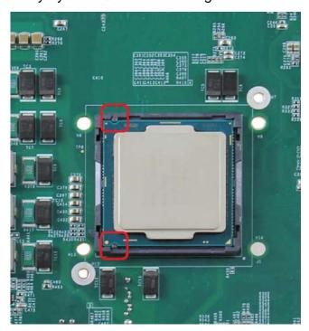
5. Get the CPU retaining bracket from the accessory box and place it on the top of CPU. The CPU retaining bracket shall be screwed from the opposite side. Please hold the CPU and bracket firmly while turning the PCBA upside down, and secure the CPU retaining bracket with two M3 P-head screws.
