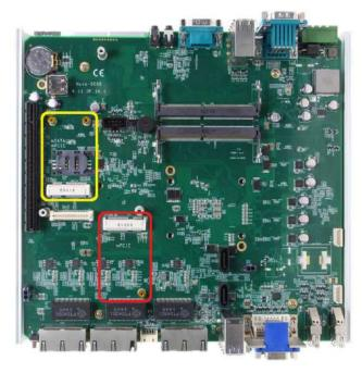
2. Tilt the mini-PCIe 3G module and insert it into the mini-PCIe #2 socket (marked as red). And fix the module with one M2.5 P-head screw.
