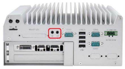
Nuvo-5095GC series provides audio function using Intel<sup>®</sup> High Definition Audio in Q170 chipset and Realtek ALC262 codec. There are two audio jacks on the back panel. The left one is used for microphone input, and the right one is used for speaker output. To utilize the audio function in Windows, you need to install corresponding drivers for both Intel<sup>®</sup> Q170 chipset and Realtek ALC262 codec. Please refer to section 4.5 for information of driver installation.
