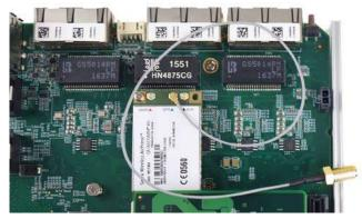
4. Fix the SMA connector of the IPEX-to-SMA cable to one of the four antenna apertures on either front panel of back panel.
