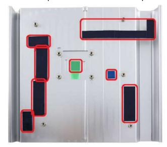
Put the PCBA back to heat-sink. Make sure all the screw holes on PCBA are aligned with mounting posts of the heat-sink.
