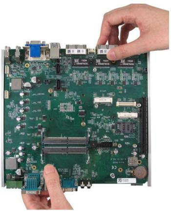
8. Get five M3 spring screws from the accessory box. Fix them according to the order indicated on the photo (red circles). And tighten four M3 P-head screws (yellow circles) to fix the PCBA to the heat-sink.
