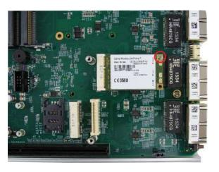
3. Attach the IPEX-to-SMA cable to the 3G module.
