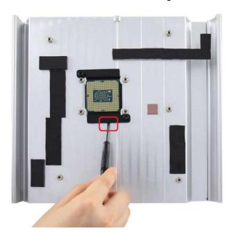
5. Check the condition of thermal pads on the heat-sink, especially the thermal pad for CPU. If it's broken, please replace it with a new one.
