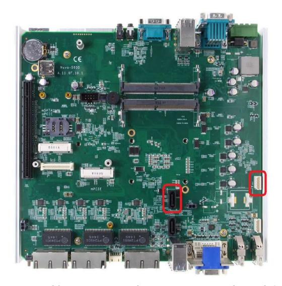
Nuvo-5095GC series provides two SATA ports which support Gen3, 6 Gb/s SATA signals. Each SATA port is composed of a 7-pin SATA connector and a 4-pin power connector. SATA port #1 is used in conjunction with the HDD bracket to accommodate the first 2.5" HDD/SSD. A dedicated cable is shipped with the system to provide standard 22-pin SATA connector. For information of installing a HDD/SSD to SATA port #1, please refer to section 3.4 for detail.
