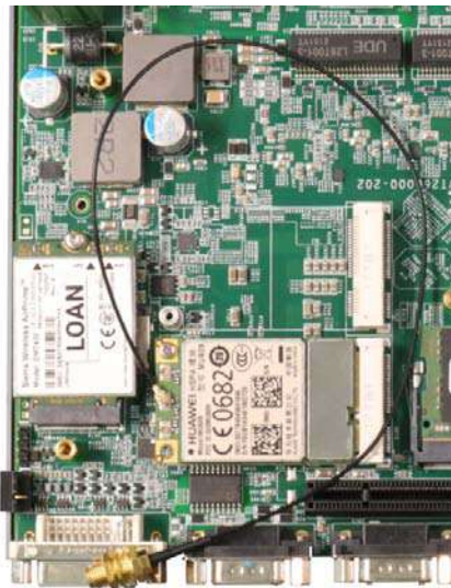
Clip on the IPEZ-to-SMA cable
