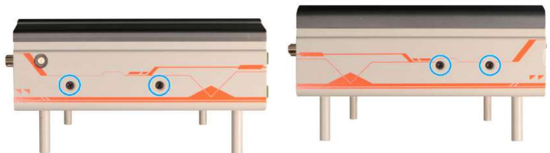
Left side chassis screws
