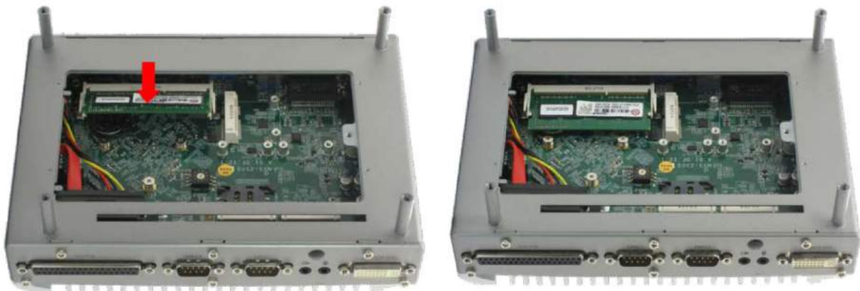
Figure 48: Install the Memory Module
