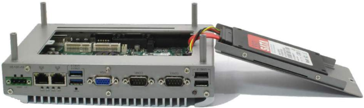
Figure 51: Connect HDD to the SATA Cable
