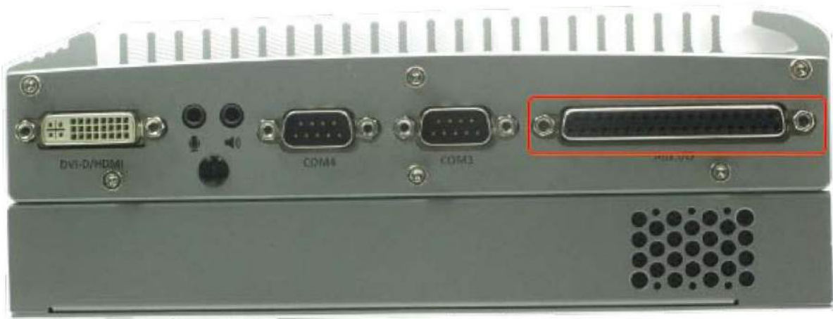
Figure 17: Auxiliary I/O on Nuvo-2500
