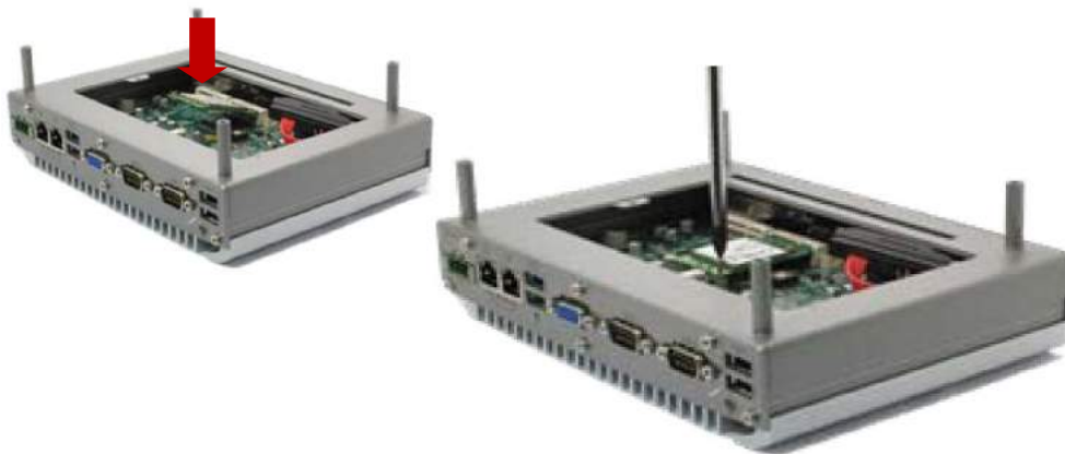
Figure 54: Install and Lock the Mini-PCle Module
