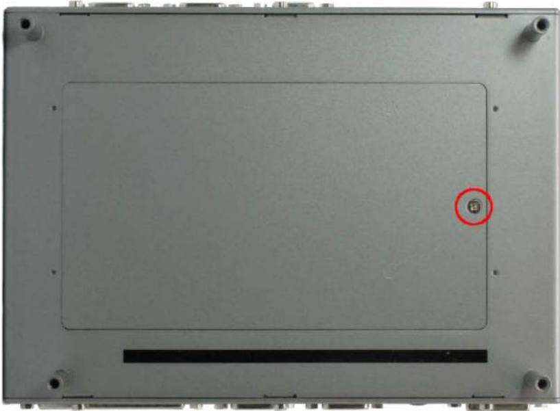
Figure 42: Nuvo-2500 and Nuvis-2520at Back Cover Screw
