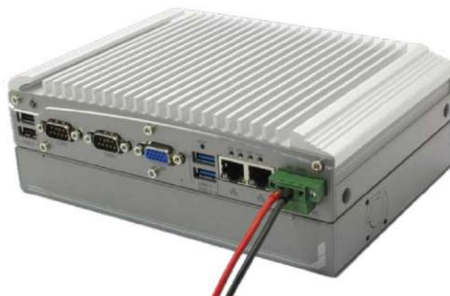
Figure 66: System with DC Input Terminal Block
