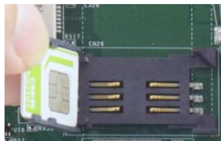
Insert SIM card with pins facing up
