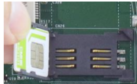
Insert SIM card with pins facing up
