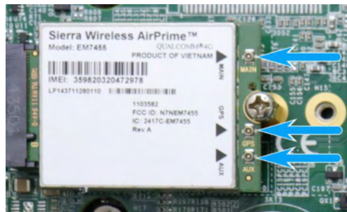
Clip on the IPEX-to-SMA cable
