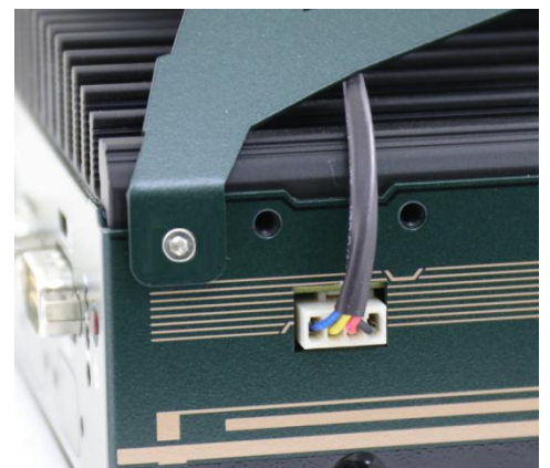
Plug in the 4-pin power connector
