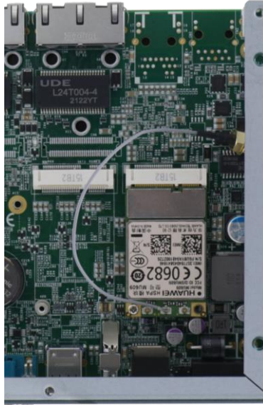
Clip on the IPEX-to-SMA cable
