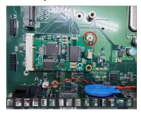
Step 5 Connect the cable to the module and assemble I/O connector to fix the I/O bracket then fasten dual screws of the Flexible I/O Window.
