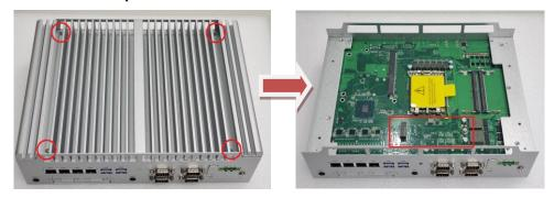
Step 4 Insert M.2 NVMe module into the slot and tighten the screw.
