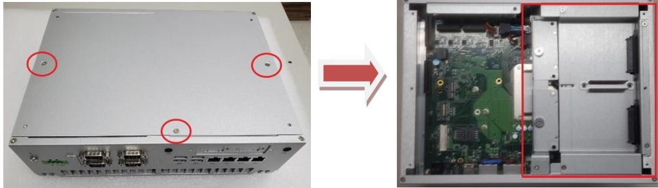
**Step 3** Assembly each SSD/HDD with the HDD bracket with 2 screws.
