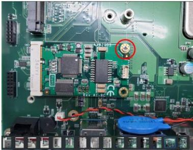
**Step 5** Connect the cable to the module and assemble I/O connector to fix the I/O bracket then fasten dual screws of the Flexible I/O Window.
