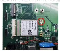
Step 5 Remove the antenna cover from system, fix the SMA connector of the IPEX-to-SMA cable to one of the five antenna apertures on either front panel of back panel.
