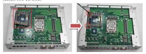
Step 5 Prepare the optional heat spreader (comes with MXM T1000 module kit) and put the grease as below red marked on the bottom side of the copper heat spreader.
