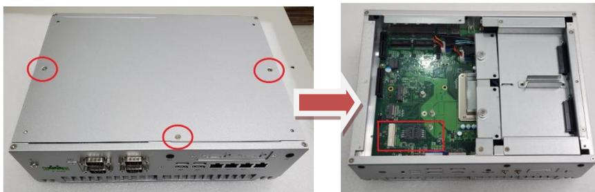
**Step 3** Insert the corresponding SIM card into SIM socket (CN22) before you install the mini-PCIe module.
