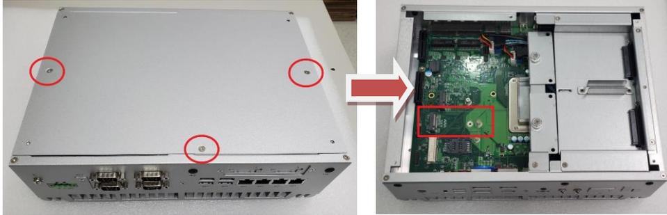
**Step 3** Insert 5G wireless module into the slot and tighten the card securely to the mainboard with M3x3 screw, and attach the IPEX-to-SMA cable to the 5G module.
