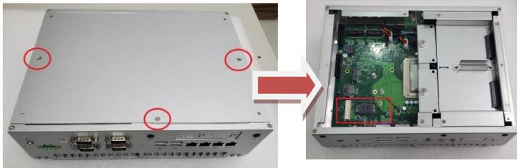
**Step 4 Insert a mini PCIe module into the socket and tighten the card securely to the mainboard with one M3x2 screw.**
