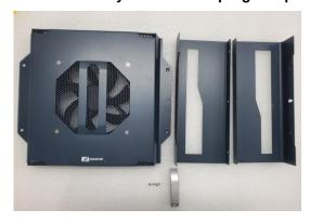
Step 3 Assemble the fan kit bracket on both side of the system first and then secure four screws as red marked.
