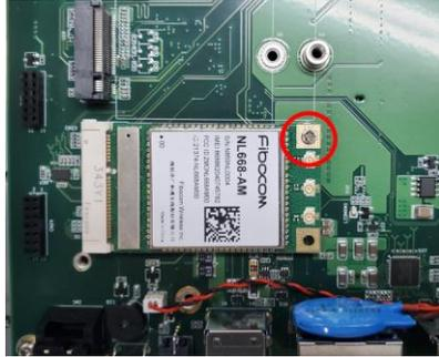
**Step 5** Remove the antenna cover from system, fix the SMA connector of the IPEX-to-SMA cable to one of the five antenna apertures on either front panel of back panel.
