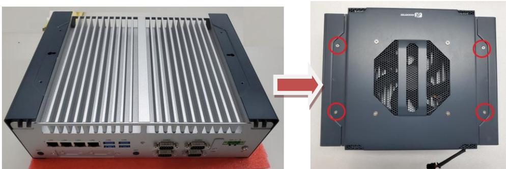
**Step 5** remove the FAN connector cover.
