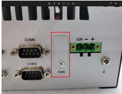
**Step 6** Connector the fan cable to the fan connector of the system and put the cover back.
