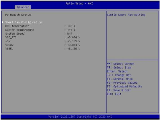
This screen displays the temperature of system and CPU as well as system voltages (VCORE, +3V STBY, +5V STBY and +5V).
