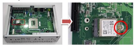
Step 4 Attach the corresponding IPEX-to-SMA cable (2pcs) to the module as below red marked.
