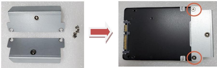
**Step 4** Push the SATA drive tray to insert the connector firmly and fasten the screw to make sure the insertion is complete.
