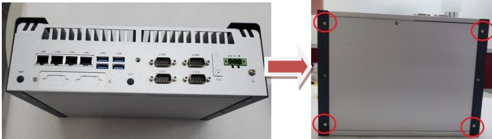
**Step 4 Put the FAN kit top cover and fasten 4pcs screws.**
