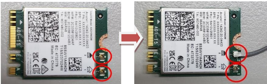
**Step 5** Remove the antenna cover from system, fix the SMA connector of the IPEX-to-SMA cable to one of the five antenna apertures on either front panel of back panel.
