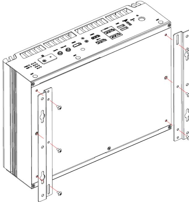
Note : If users install the screws in drywall, use the hollow wall anchors to ensure that unit does not pull away from the wall due to prolonged strain between the cable and power connector.
