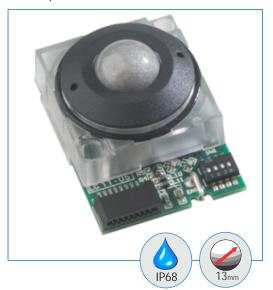
Utilizing the latest and most advanced laser tracking technology, the X13 laser Trackerball™ is an extremely high specification, contact-less device, ideal for the most demanding of cursor control applications.
