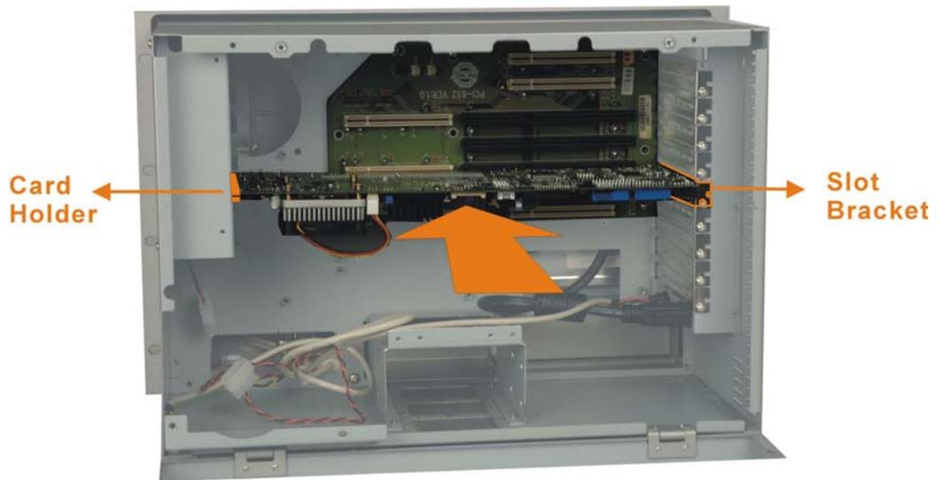
**Figure 2-5: CPU Card Installation**
