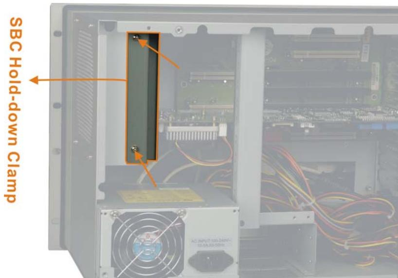
**Figure 2-8: Installing the SBC Hold-down Clamp**
