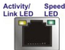
**Figure 3-12: RJ-45 Ethernet Connector**
