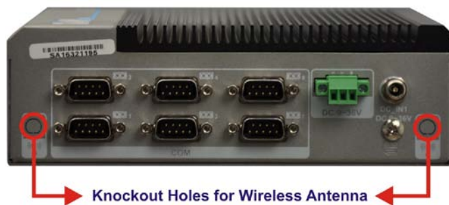
Figure 3-4: Knockout Holes for Wireless Antenna
