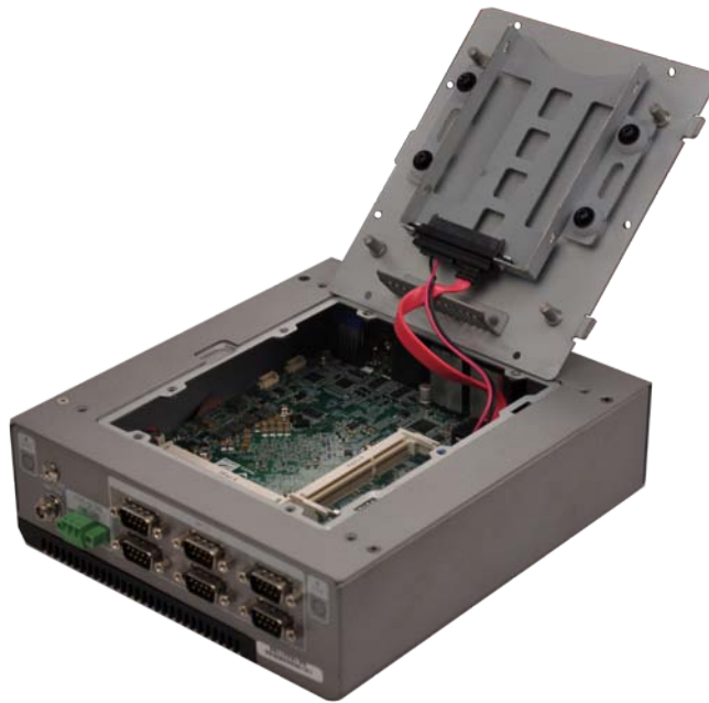
Figure 3-2: HDD Bracket Retention Screws
