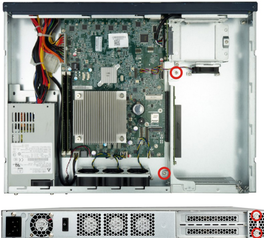
Figure 3-6: Expansion Slot Module Retention Screws
