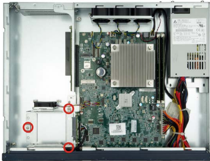
Figure 3-3: HDD Bracket Retention Screws
