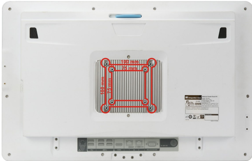
Figure 3-27: VESA 75 and VESA 100 Mounting Retention Screw Holes
