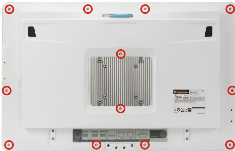
Figure 6-1: Back Cover Retention Screws
