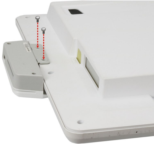
Figure 3-17: Combo Reader Installation
