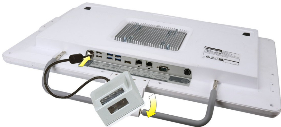
Figure 3-12: Install and Connect Barcode Reader Set
