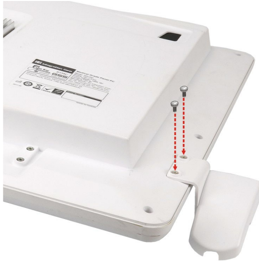
Figure 3-4: Handset Holder Retention Screws
