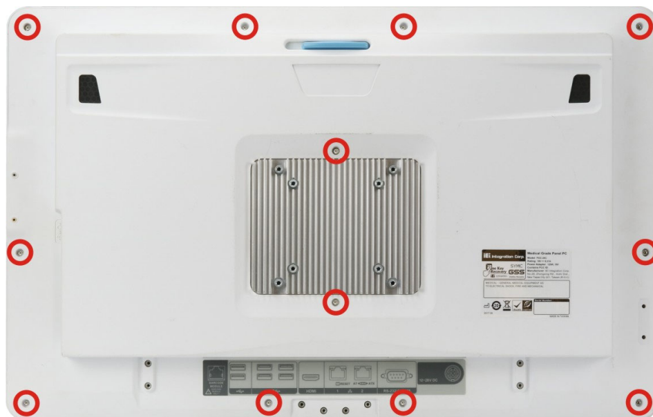
Figure 3-1: Back Cover Retention Screws
