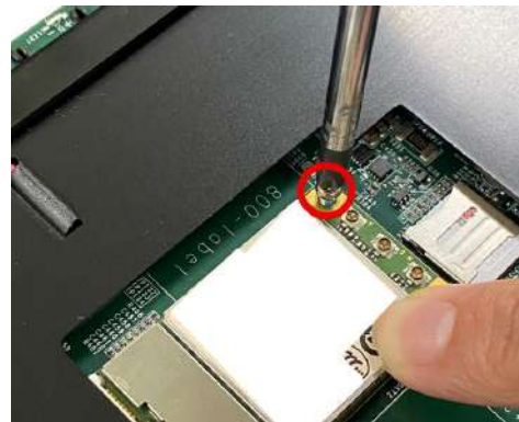
Secure the card with a screw
