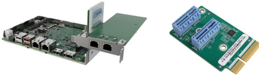
Figure 4-4: Outwards Riser Card Installation Example Figure 4-5: NWR-L2S-N-R10
