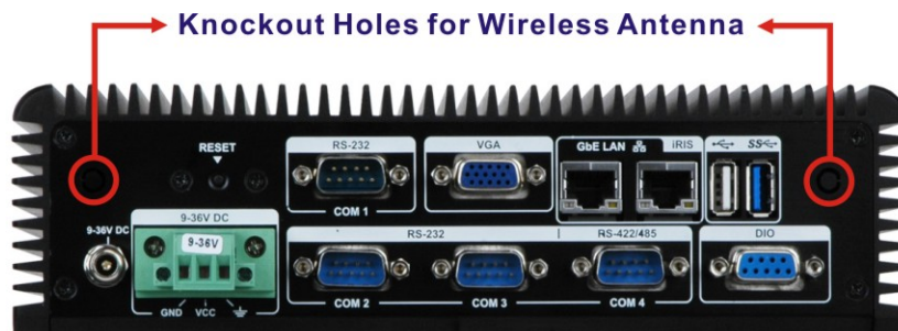
Figure 3-16: Knockout Holes for Wireless Antenna
