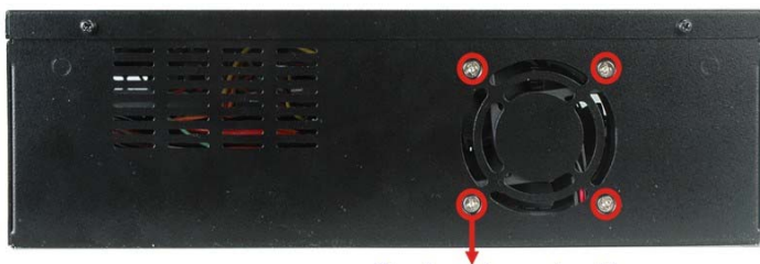
System fan retention screws
