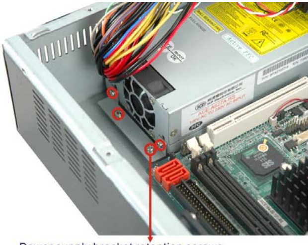
Power supply bracket retention screws
