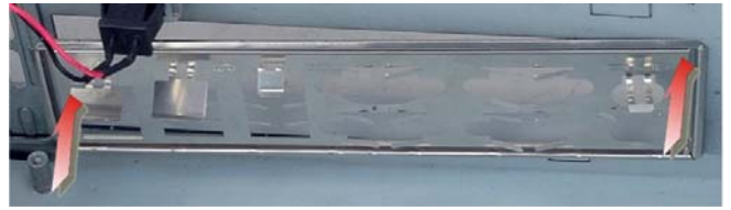
Figure 5: I/O Bracket Installation
