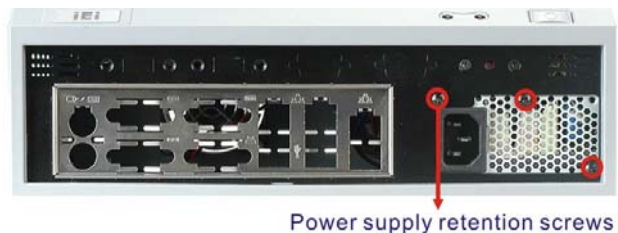
Figure 13: Power Supply Retention Screws
