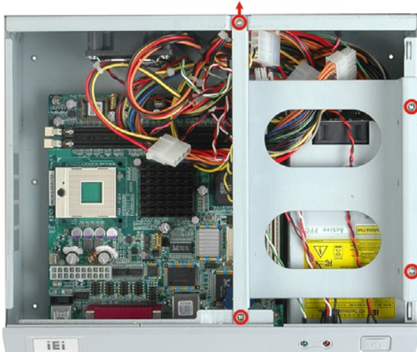
Figure 4: HDD Bracket Retention Screws
