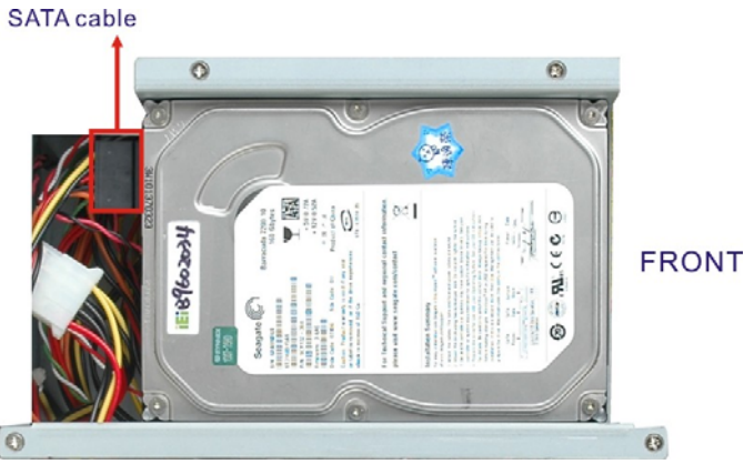
Figure 7: HDD Bracket (Top)
