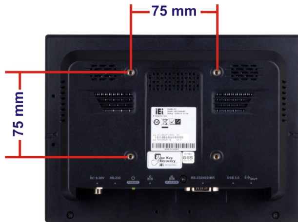
Figure 3-21: Arm Mounting Retention Screw Holes
