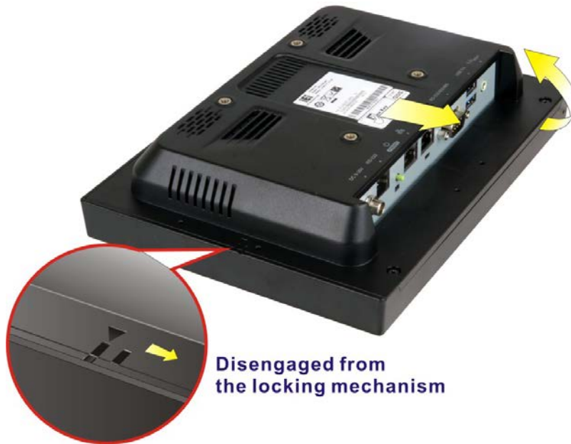
Figure 3-2: Remove the Back Cover
