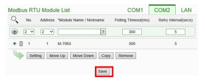
Please note: if fail to scan the I/O modules, please make sure the RS-485 cable is properly connected. And then go to Step 1: "System Setting" $\rightarrow$ "I/O Interface Setting" to make sure the settings of the COM Port that are connected to the I/O Module are accurate. After all settings are completed, click "Save" button to save the changes and repeat Step 3.a to perform scanning of the I/O modules again.
