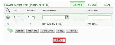
Please note: if failed to scan the power meters, please make sure the RS-485 cable is properly connected. And then go to Step 1: "System Setting"  $\rightarrow$  "I/O Interface Setting" to make sure the settings of the COM Port that are connected to the power meter are accurate. After all settings are completed, click "Save" button to save the changes and repeat Step3.a to perform scanning of the power meters again.
