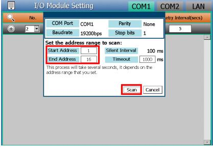
c. After the Scan operation is completed, an M-7000 I/O module list will appear. After all settings are completed, click "Apply" button to save the changes.
