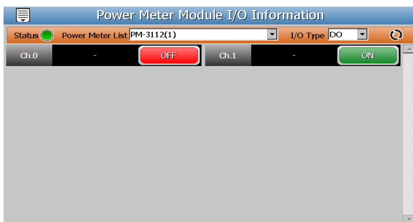
Figure6-1: Power Meter I/O channel Status
