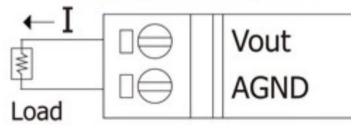
I-8024W Current Output Wiring
