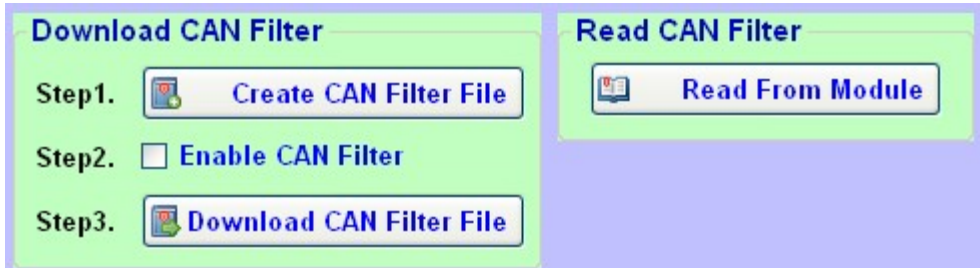
Figure 4-3 Set and read the CAN filter configuration
