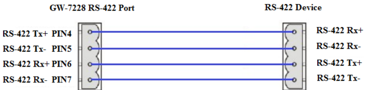
Figure 2-6: RS-422 Wire Connection
