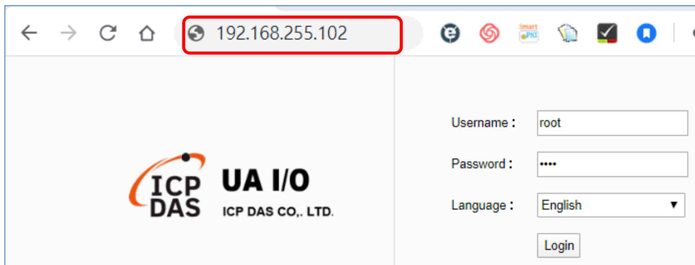
Figure 36 2-2-1 Use the new IP to login the Web UI of UA I/O
