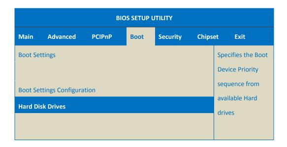
Step 5: Set 1st Drive as PS-xxx, it means the XP-8000-Atom booting from the CF card
