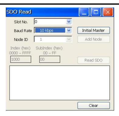
Step 6: Assume the I-87123 is plugged in slot 0 of the WinPAC, and the baud of the CANopen network is 1000 kbps, set the "Slot No." and "Baud Rate" as following figure. Then click "Initial Master" to initialize the I-87123.
