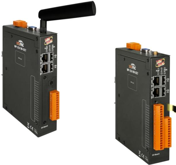
The WP-2241M-CE7 are equipped a Cortex-A8 CPU (1 GHz) and running a windows CE.NET 7.0 operating system. The optional I/O expansion board, XV-board, provides high-protection I/O. Using the built-in Flash and microSD, the WP-2241M-CE7 can save application program, image file and data.
