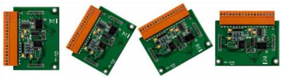
WP-2241M-CE7 is equipped with an I/O expansion bus to support one optional expansion board, called XV-board. It can be used to implement various I/O functions such as DI, DO, A/D, D/A, Timer/Counter
