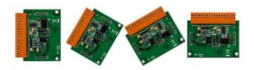
WP-2241M-CE7 is equipped with an I/O expansion bus to support one optional expansion board, called XV-board. It can be used to implement various I/O functions such as DI, DO, A/D, D/A, Timer/Counter
