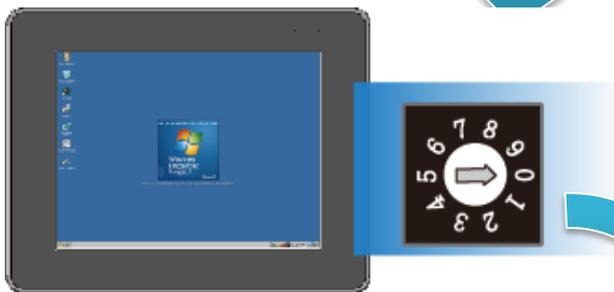
**Step 6: Turn the rotary switch in position 0, normal mode**
