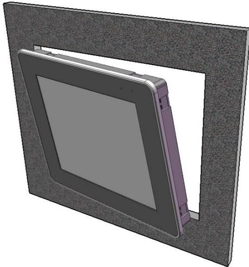
**Step 3: Insert the panel mounting clips into the upper and lower ventilation holes**
