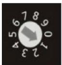
Rotary Switch is an operating mode selector. The VP-X201-CE7 has several operating modes, for more detailed information about these operating modes. Please refer to “2.3 Configuring the Boot Mode”
