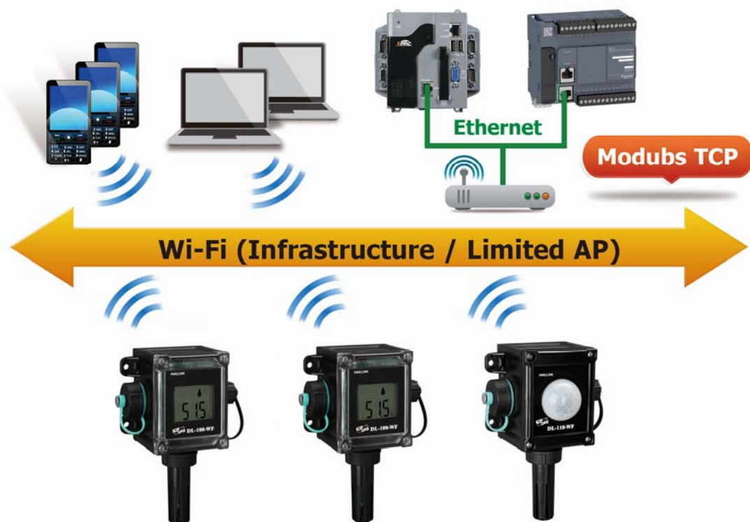
Figure 1-1: Application architecture for the DL-1xxS-WF
