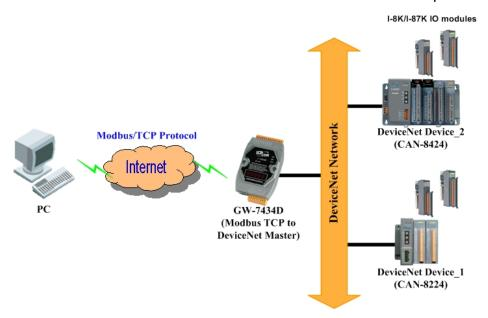
After configuring and letting the GW-7434D start to communicate with these two DeviceNet devices by Utility tool, users can get the data of these two devices via communicating with the GW-7434D with Modbus TCP protocol.
