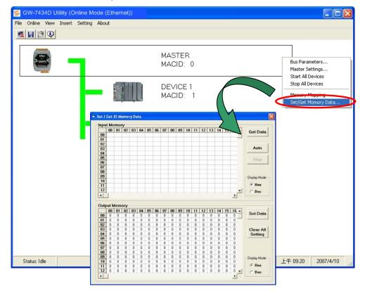
**Step2:** Users can get the Device1, 2 bytes polling input data, and Device2, 16 bytes polling data, on the Input Memory Table, 0000~0001 and 0100~0115 after click the "Get Data" button or "Auto button".
