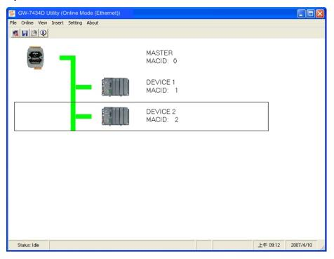
**Step7**: Finally, users need to map these two devices' IO connection data path into GW-7434D's Input/Output Data Area. So that users can get/set IO data from/into IO Data Area via Modbus/TCP function 16 command, force multiple registers, to get/set these two DeviceNet devices' IO data.
