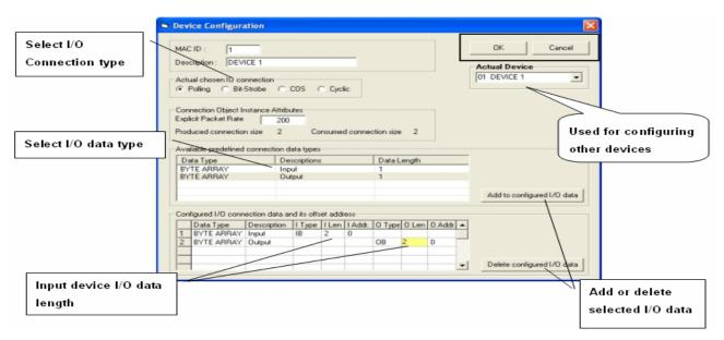
**Step6**: After configuring these two devices, the GW-7434D will start to communicate with two devices. And the Utility will start to monitor the status of the GW-7434D.
