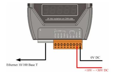
**Step3:** Connect the Ethernet ports of the GW-7434D and the PC to the hub with standard network cable respectively.
