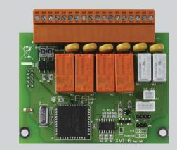
XV116 5-channel Isolated Digital Input and 6-channel Relay Output Module
