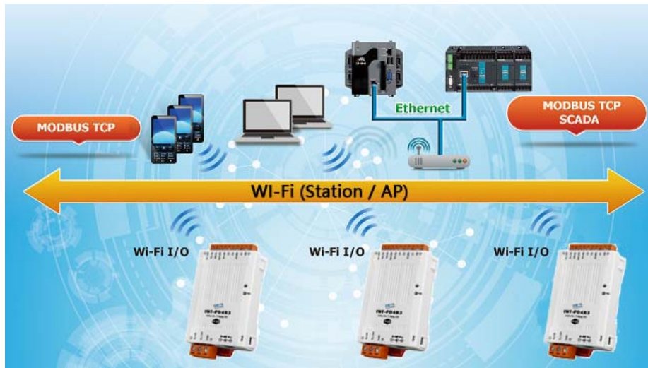
Figure 1-1: Application architecture for the tWF series
