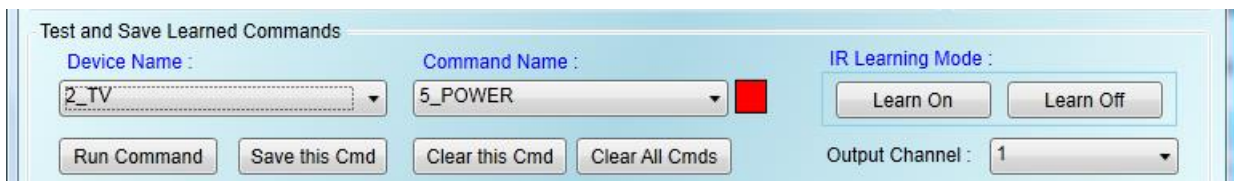
▲ Figure 3-14 Test & save learned IR commands section.
