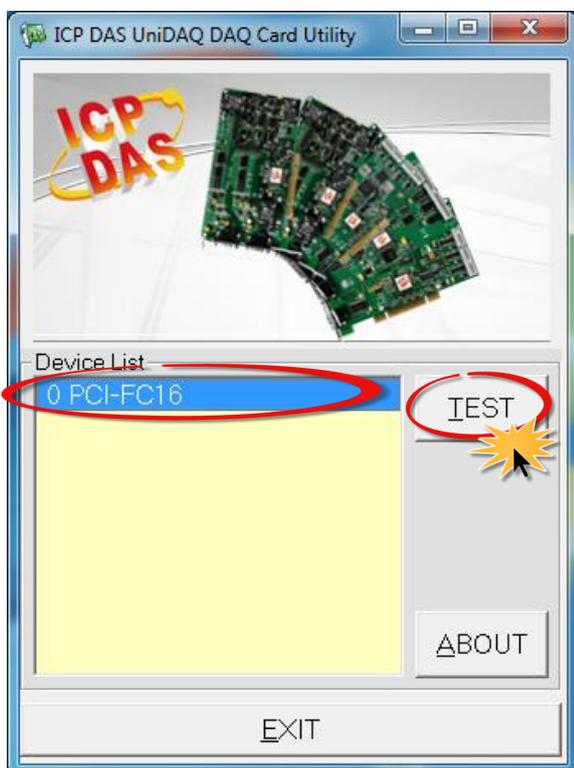
**Step 2:** Confirm that the PCI-FC16U board has been successfully installed in the Host system. Note that the device numbers start from 0.
