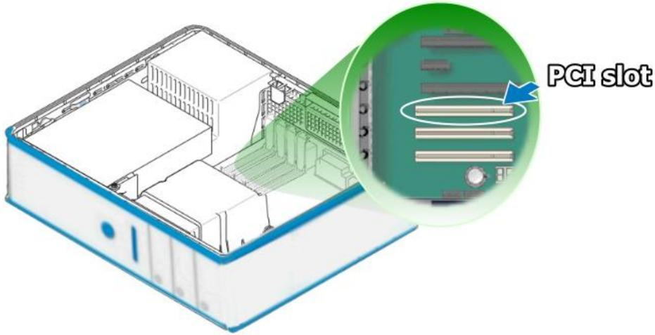
Step 6: Unscrew and remove the PCI slot cover from the computer case.
