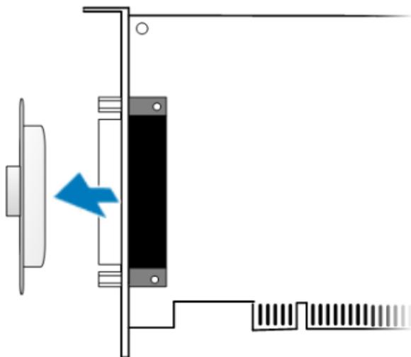
Step 7: Remove the connector cover from the PCI-FC16U board.
