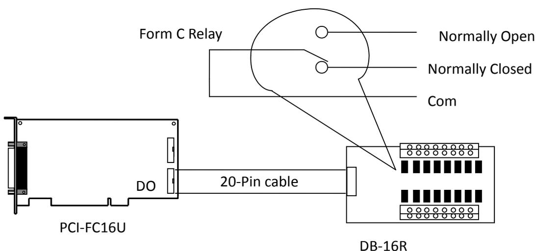
*Note: Relay controls load up to 0.5 A @ 110 V<sub>AC</sub> or 1A @ 24 V<sub>DC</sub>*
