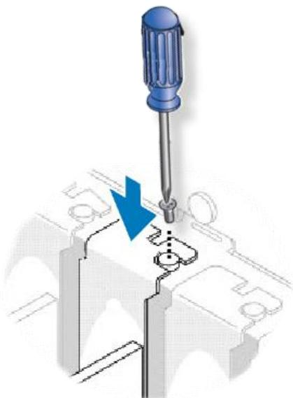
Step 9: Confirm that the card is correctly inserted in the motherboard, and then secure the PCI-FC16U board in place using the retaining screw that was removed in Step 6.
