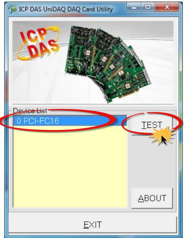
**Step 6:** Check the results of the **Digital Input/Output** functions test.
